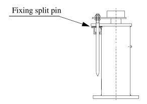
For the extention of the oil buffer remove the split pin, pay attention to the upper movement of the oil buffer ram.
